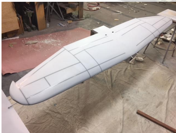
Franks P-47 Wing, Rivets and Panel Lines Ready to Prime
